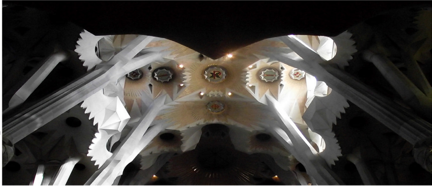
Fig. 3 - Hyperboloid of revolution of one sheet (Diagram on the left in exhibition "Formas e Fórmulas" MUHNAC, Lisboa, April 2014) applied on nave, Sagrada Família, Barcelona.
