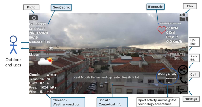
FIGURE 5. Middleware layout example. Informative elements are indicated by the blue boxes, system-related elements by white boxes, and functional elements by the grey ones.
