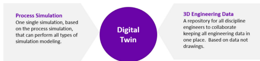
FIGURE 5.4. Digital Twin components in engineering [19]
