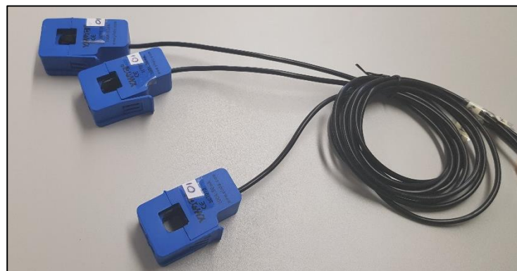
Figure 4 - Three TC SCT-013-000 Sensors used to measure three-phase current.
