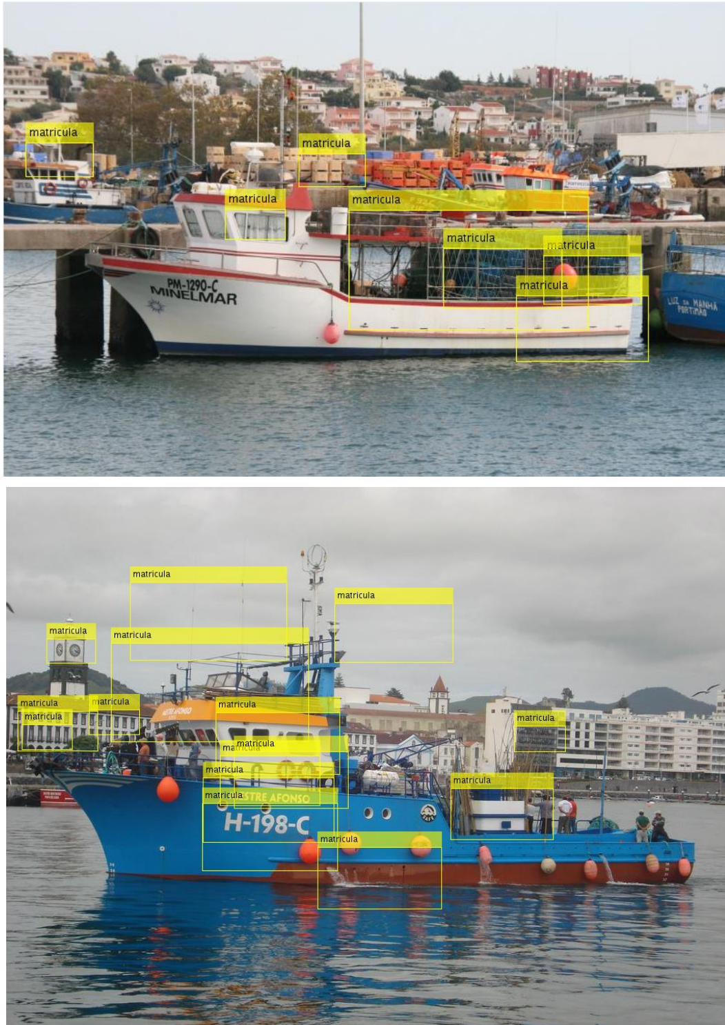
Figure 23 – Result of the application of an LBP classifier, trained with False Alarm Rate of 0.5 and 20 stages completed.
