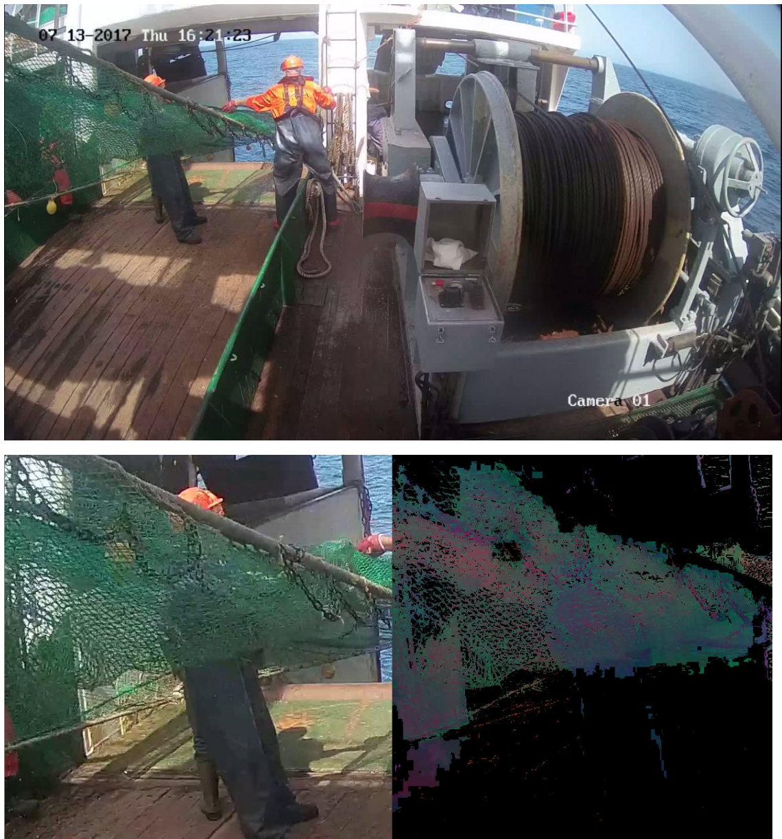
Figure 38 – Application of the algorithm in the input image (above) and corresponding results with segmentation (right) and without segmentation(left)
