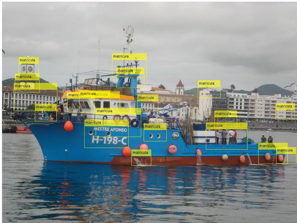
Figure 24 – Result of the application of a HOG classifier, trained with False Alarm Rate of 0.5 and 20 stages completed.
