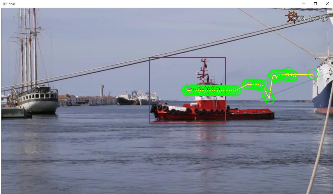
Figure 17 – Output displayed after running the algorithm on a video. In green are represented the centroids of the object for each frame processed, and yellow, to join the centroids, the estimated path covered by the object.
