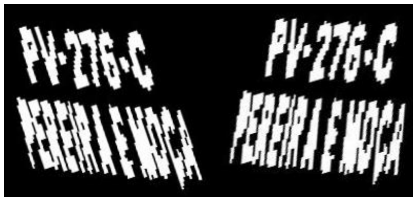
Figure 35 – Result after operation of rotation (left) and after deskew (right) using the forth approach
