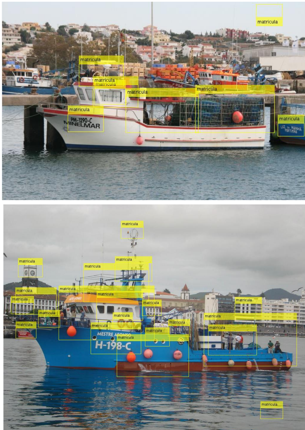
Figure 22 – The result of the application of a Haar cascade classifier, trained with False Alarm Rate of 0.5 and 20 stages completed.
