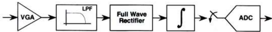
Fig. 6.8 – Area detect servo burst demodulator architecture.
