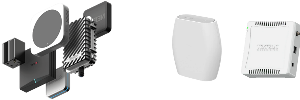
Figure 3.3: Helium hotspots (left) and The Things Network gateways (right) for grating LoRa network coverage in areas with low coverage.
