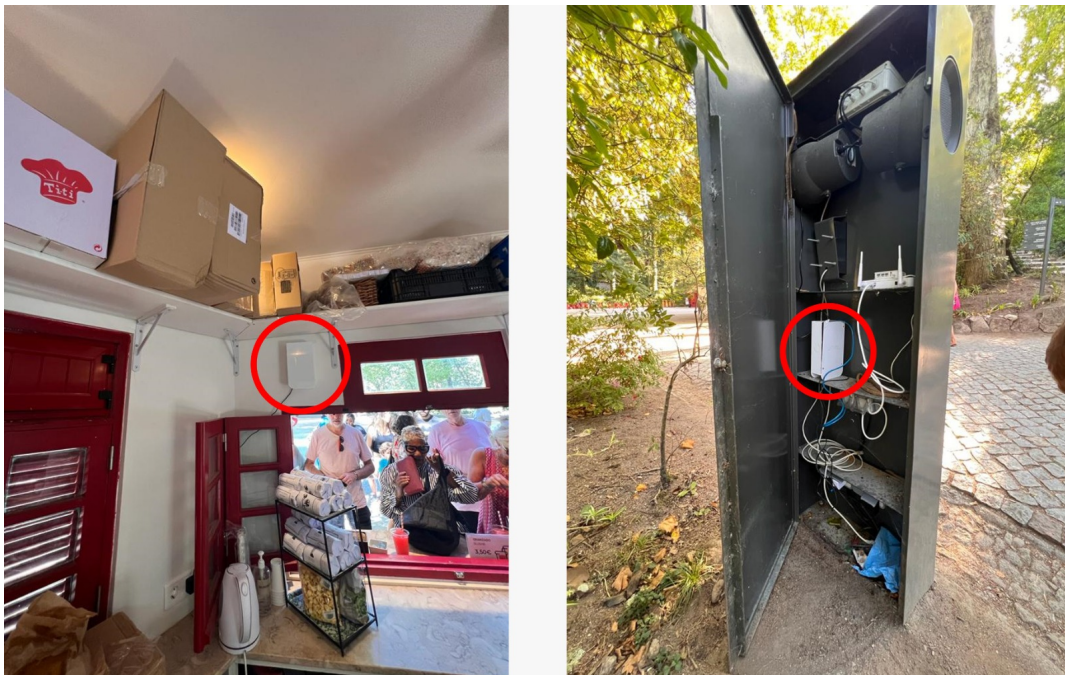
Figure 5.13: Deployment of sensors in Picadeiro's Kiosk (left) and inside a Help-point (right).
