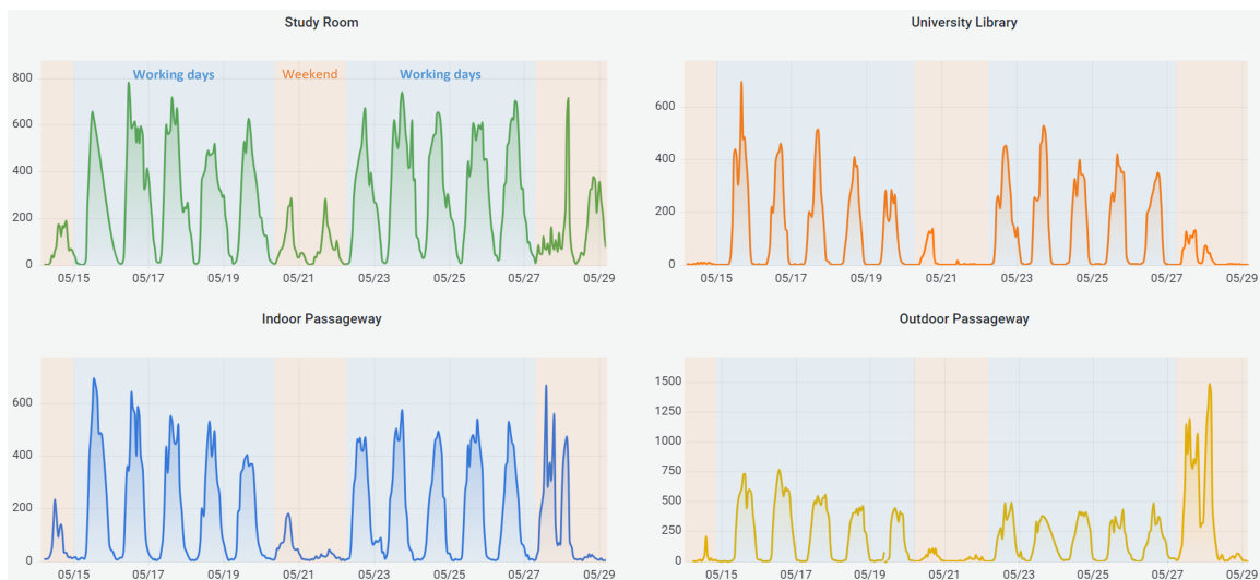
Figure 5.2: Dashboard with a collapsed view of each sensor deployed at Iscte's Campus in a two-week period. The working days are filled in blue, and the weekends are filled in orange.
