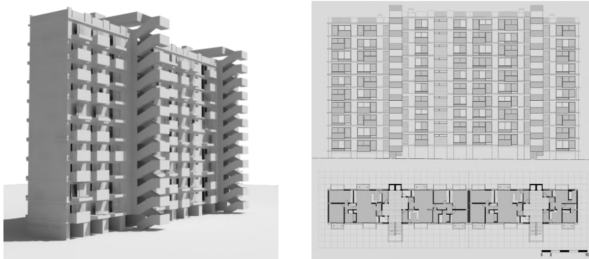
Fig.14. 3D View, Main Facade, Plant of proposed eight-story blocks. FSC, ILR, Atelier , Queijas, Work session 27.09.2018
