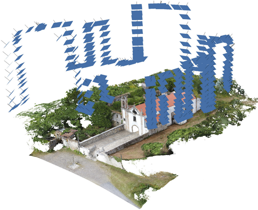
Fig. 8 – Photogrammetric survey of the convent carried out by UAV, with the indication of the acquisition points. ©Roberta Ferretti, 2021.
