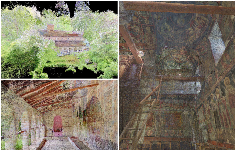
Fig. 7 – Point cloud from Laser Scanner: the main facade, the portico and the interior of the church. ©Francesco Tioli, 2019.
