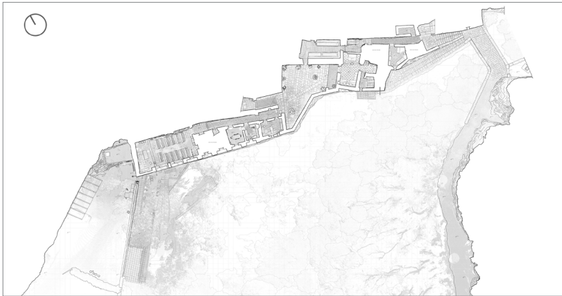
Fig. 3 – Plan of the ground floor of the Eremo delle Carceri, elaborated starting from the digital survey carried out with laser scanner instruments. ©Carlotta Assirelli, 2021.
