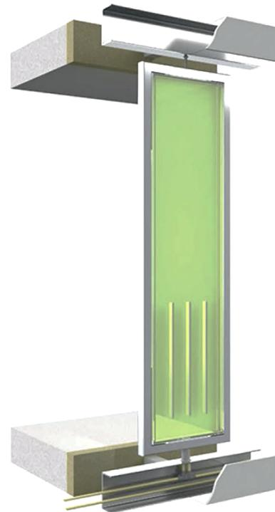
The bioreactive facade – principle construction methodology of the SolarLeaf
