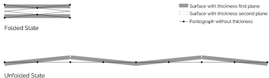
Figure 4.33. prototype C folding states for Scissor Elements design
