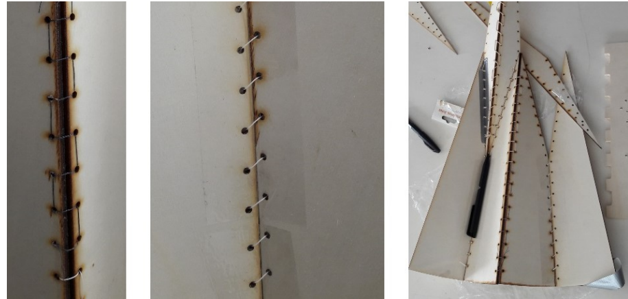
Figure 3. 102. Experiment 03 Group C - Plywood Stitching
