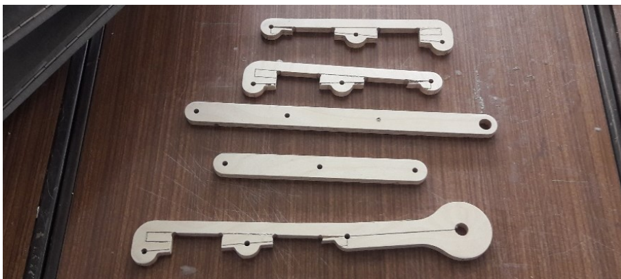
Figure 4. 53. Final pantograph pieces
