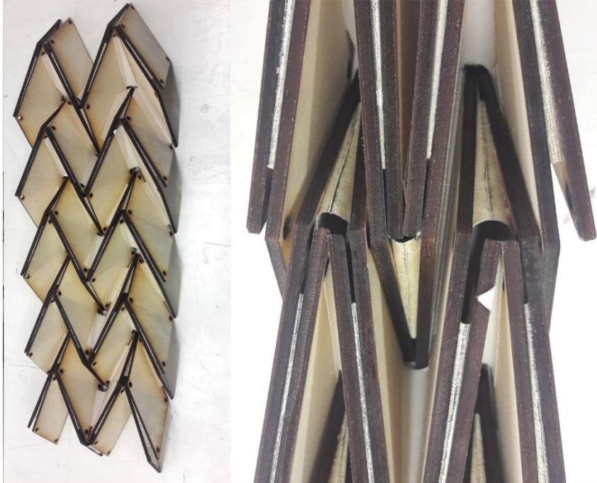
Figure 3.70. Miura tessellation with plywood rigid faces using the Axis Shift Method
