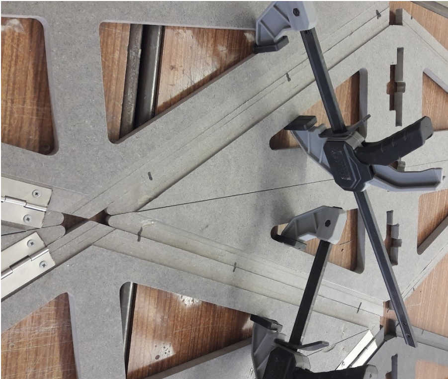
Figure 4. 43. Voids for screws and bolts and low relief for piano hinges
