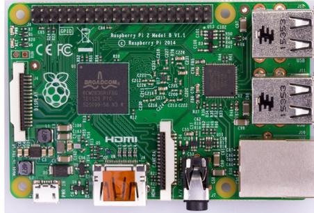
FIGURE 2.8: Raspberry pi 2 Model B. The same board as used during the development of this project.
