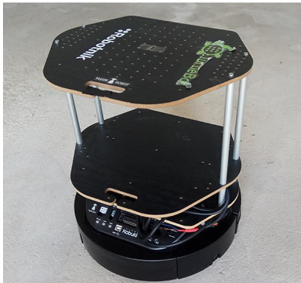
FIGURE 2.5: Turtlebot 2. The robot used on this project.
