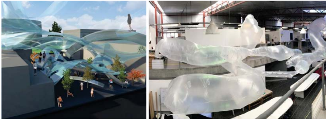
Figure 9. Projects 3 & 4 combined: Inflatable layer above the ground offers alternative ways to occupy the urban setting. Prototype structure adapted and fabricated at natural size at the studio space (Alley, A., De Belle, B., Reyes Castillo, N.A., Triantafyllou, C., Re-morphing the Amorphous , 2016).
