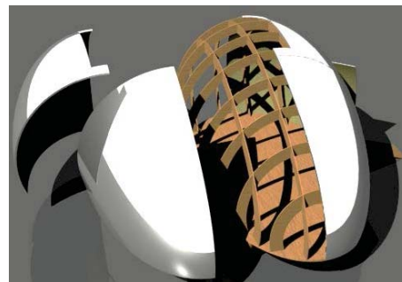
Figure 7. Final module's 3D modulation: Extruded aluminium plaques
