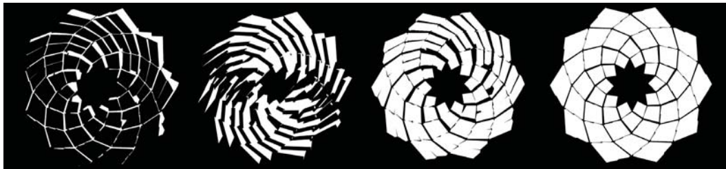
Figure 4. Shadow Impact - These images show the level of impact from shadows based on the orientation of the surfaces. The white is the shadow coverage. On the far left are the shadows from a horizontal position suggesting a summer condition with high sun exposure, on the right are the shadows shown from a vertical position suggesting either a cooling condition or optimizing for low winter sun exposure.
