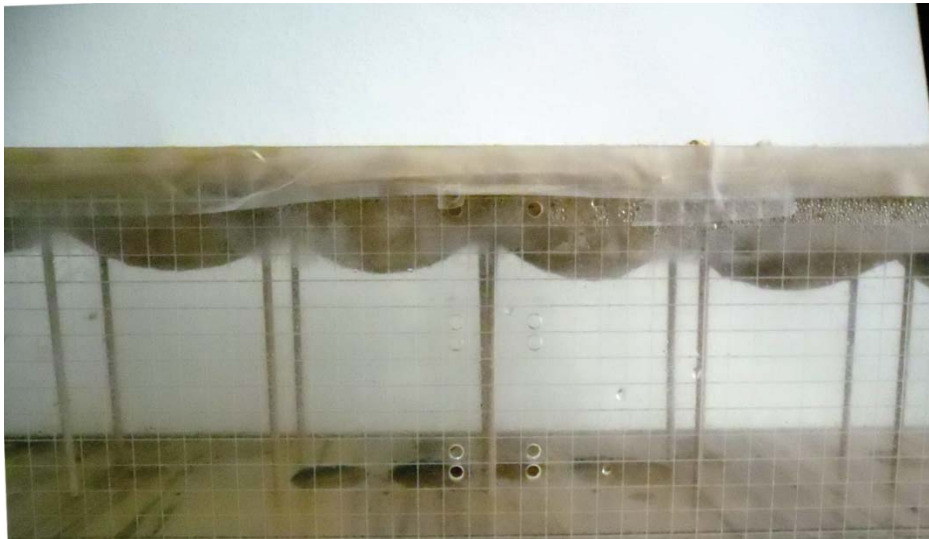
Figure 7. Fluctuation on the MbM shape due to irregular distribution of dead load (Initial shape).
