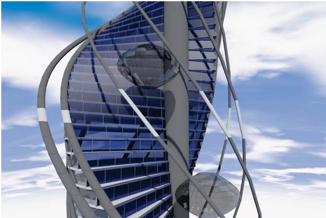
Figure 5. Highlighted columns (in white) from Wadala's façade skin
