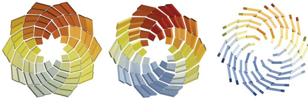
Figure 3. Solar Radiation and rotation) Rendering series showing simulated exposure and surface rotation from a horizontal bed to a vertical position.
