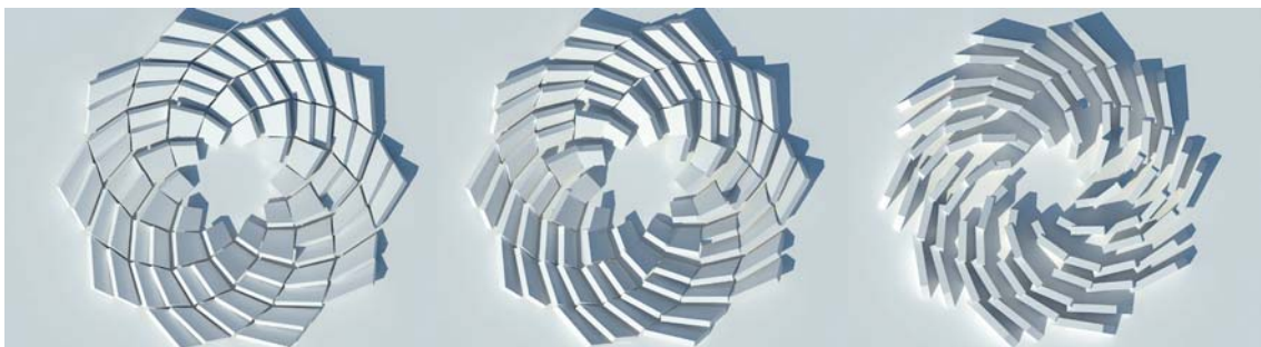
Figure 2. Conceptual Movements - Heliotropic Prototype Design) Renderings showing design of the prototypes movements throughout the day, from a horizontal position on the left, towards a shaded vertical condition on the right. Shown above are unified movements to convey the angle change. Actual suggested movements would be based on local indicators and individual rotations of beds.
