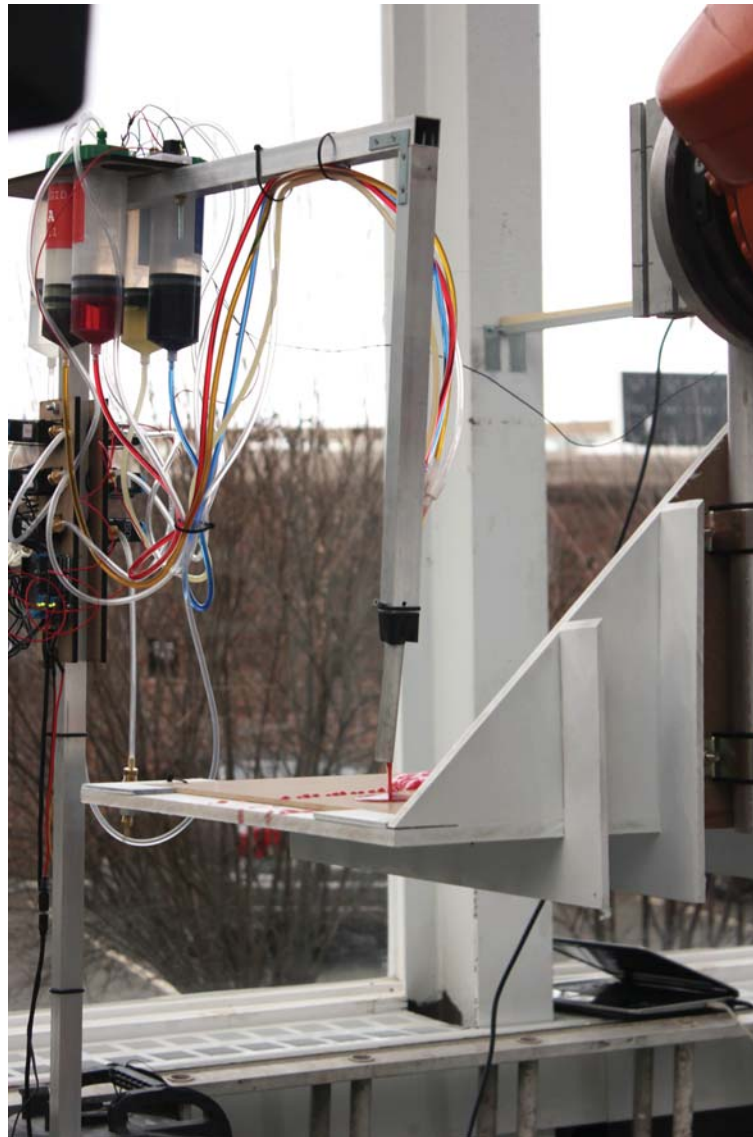
Figure 4. Foam Deposition in Progress.
