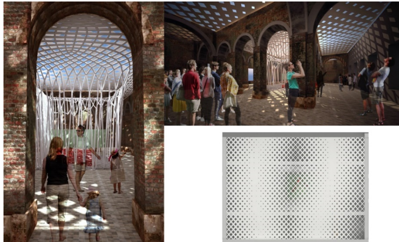
Figure 8. The effect of the perforated shading device in manipulating with the natural daylight and the shadow that have been created in the space, adding to allow more natural ventilation using outdoor thin fabrics like ETFE. Author work
