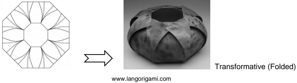
Figure 1. The Additive, Subtractive and Transformational Methods of making objects. Folding is unique because it neither adds nor subtracts materials during the process of making, but transforms them.
