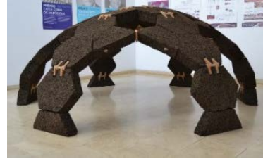
Figure 12 – Cork used as a self-supporting material
