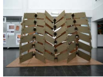
Figure 15 – Cork used as a self-supporting material
