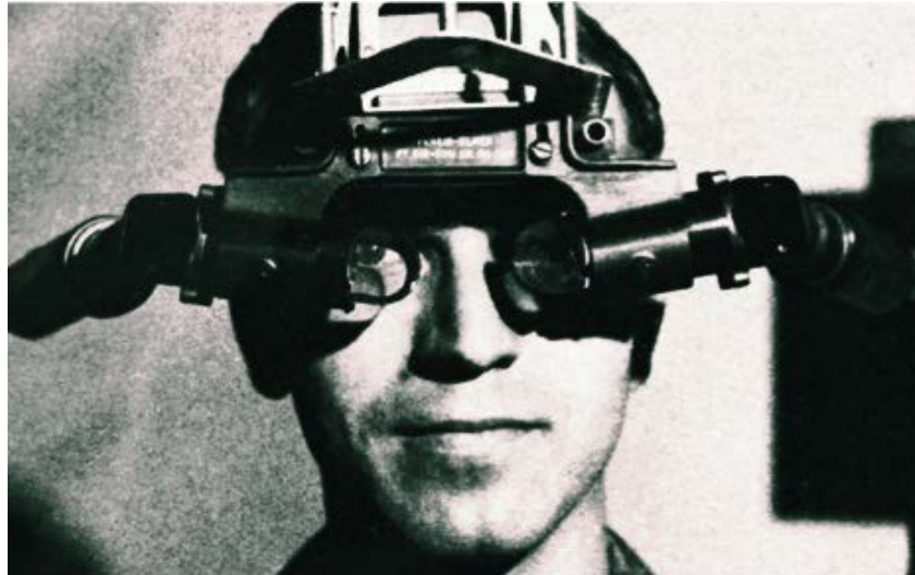
Figure 1. Sword of Damocles-Augmented reality headset developed in 1968
