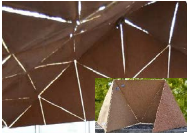
Figure 13 – Cork used as a membrane
