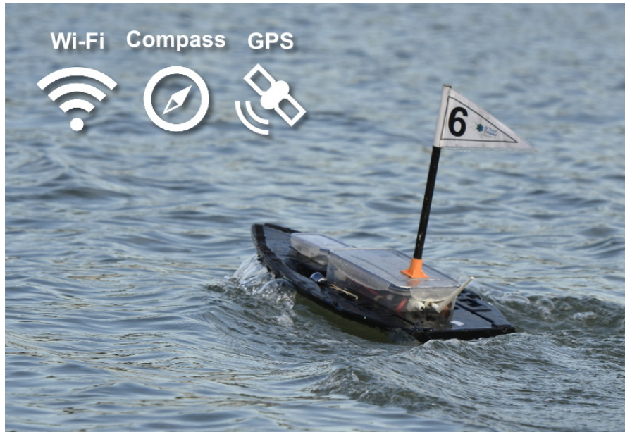
FIGURE 5.2: The robot is an autonomous surface vehicle equipped with Wi-Fi for communication, and a compass and GPS for navigation. It has a length of 60 cm and can move at speeds of up to 1.7 m/s.
